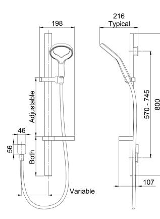
CONSTRUCTION: Brass & ABS SUPPLY: Suitable For High Pressure Systems INLET CONNECTIONS: ¼2" BSP WORKING PRESSURES: 1.0 - 5.0 bar CARTRIDGE/VALVE TYPE:N/A
