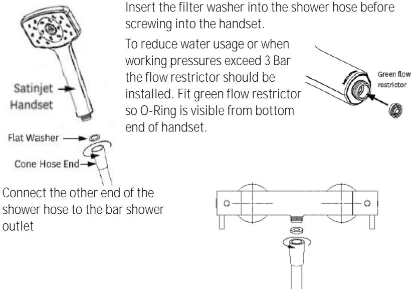
Place the handset into the handset holder of the shower rail kit. Ensuring the bar shower mixer is in the off position, turn on both hot and cold water supplies and check for leaks.
