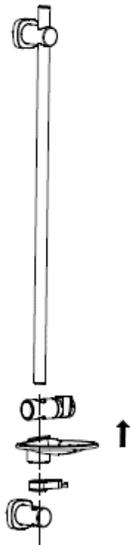
Assemble the slider, soap dish and hose retainer to the rail.
