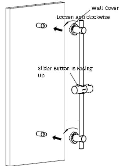
Ensuring the slide button is facing upwards as shown in the illustration, adjust and align the two wall brackets to match the position of the wall plates. Turn the wall covers anticlockwise to unlock.
