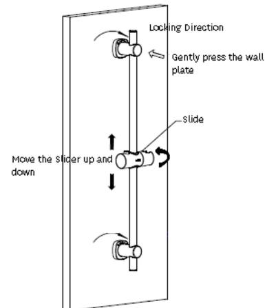
Gently press the wall brackets onto the fixing plates then turn wall covers clockwise into the locking position, securing the rail to the wall.
