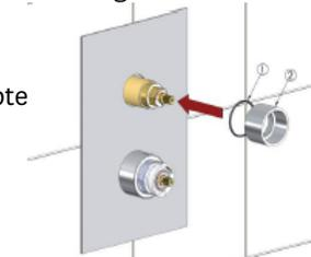
15. Refit and secure the diverter control knob and temperature knob to the position it was removed in point 11
