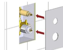
13. Fix the concealing plate on the chromed ring and on the threaded rod.
