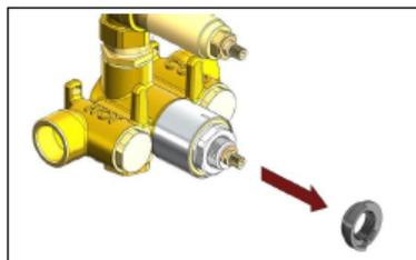
2. Unscrew the thermostatic cartridge anticlockwise with a 30mm wrench.
