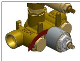
2. Remove the valve holders and clean the filters under running water or leave them soak in vinegar in presence of limescale
