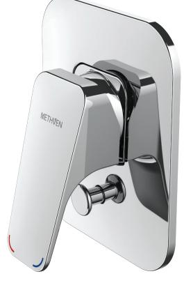
CONSTRUCTION: Brass body CARTRIDGE: Ceramic CLASSIFICATION: Suitable for mains pressure only INLET CONNECTIONS: 1/2 " BSP Male OUTLET CONNECTIONS: 1/2 " BSP Male OPTIMUM PRESSURE: 150 - 1000KPa OPERATING TEMPERATURE: 5 °C - 80 °C
