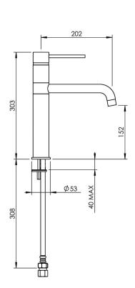
CONSTRUCTION: Brass body CARTRIDGE TYPE: Ceramic (SP033510) CLASSIFICATION: Suitable for all pressure systems INLET CONNECTIONS: 1/2 " BSP Female WORKING PRESSURE: 35 - 1000kPa DIMENSIONS FOR FITTING: 35mm diameter hole OPERATING TEMPERATURE: 5 °C - 80 °C WATER FLOW RATE: 8.0 l/pm
