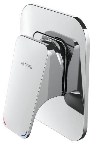
CONSTRUCTION: DR (Dezincification Resistant) brass body **CARTRIDGE**: 47 mm ceramic cartridge with Hyperflow<sup>™</sup> technology CLASSIFICATION: Suitable for equal low systems **INLET CONNECTIONS:** 1/2 " BSP Male OUTLET CONNECTIONS: 1/2 " BSP Male OPTIMUM WORKING PRESSURE: 25 - 500kPa
