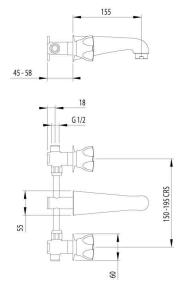
CONSTRUCTION: Brass body **CLASSIFICATION:** Suitable for **all pressure** systems **INLET CONNECTIONS:** 1/2 " BSP Male WORKING PRESSURE: 10 - 500kPa OPERATING TEMPERATURE: 5 °C - 80 °C
