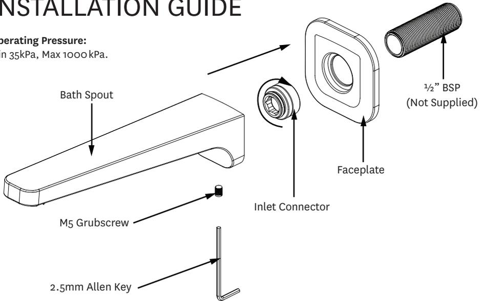
NOTE: Maximum hole diameter through wall for 1/2" BSP tube is 22mm.
