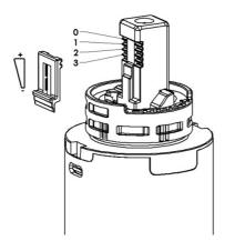
Reinsert it in to a lower groove on the stem ensuring it is fully clicked in. The handle cannot be assembled unless it is inserted correctly.
