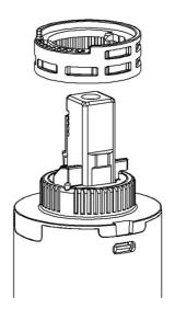
Turn the Temperature limiting ring clockwise (+) to increase maximum hot temperature, anti-clockwise (-) to reduce the maximum hot temperature.
