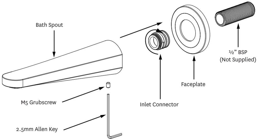
NOTE: Maximum hole diameter through wall for 1/2" BSP tube is 22mm.
