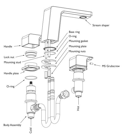
All pipework must be thoroughly flushed prior to the installation of the mixer. Inline filters must be fitted on both hot and cold supplies to prevent foreign particles damaging the ceramic cartridge.
