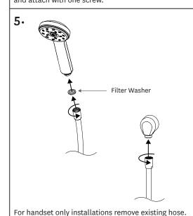
Insert the filter washer into the new hose before
