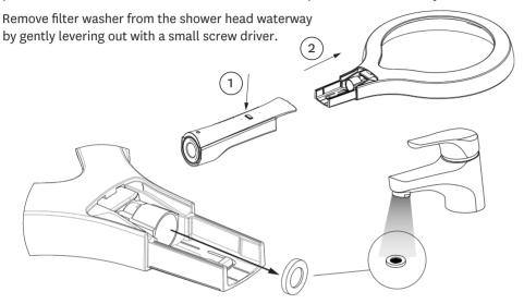
If shower performance is compromised by the build-up of lime-scale, soak in limescale remover for up to 10 minutes. Refer to instructions above for how to remove shower head from wall arm. Do not use products containing chlorine bleach or hydrochloric acid as these can damage the shower. Always rinse the shower thoroughly after cleaning to remove cleaning products that can damage the shower.
