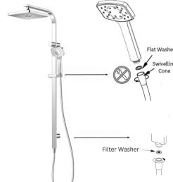
Make sure a washer is in both ends of the shower hose. Screw one end of the hose to the bottom of the shower rail, attach handset and place firmly in holder.
