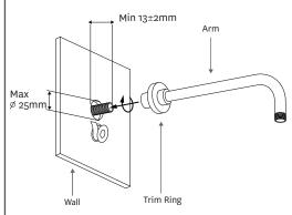
Slide chrome trim ring onto the appropriate end of the arm. Ensure that a minimum of  $13\pm2$ mm of 1/2" connection thread protrudes past the finished wall. Simply screw the arm onto the connection. Correct water proofing must be applied.
