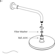
Remove the protective cap from the showerhead ball joint and screw the unit onto the overhead arm ensuring the filter washer is in place.
