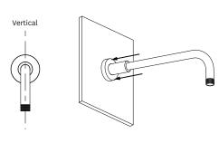
Position the arm vertically and push trim ring into place. Use wrenching flats to tighten.
