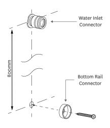
Screw the bottom rail connector to a wall stud making sure it is vertically in line with the top rail connector. Maximum centre distance between the top and bottom shower connections is 800mm.
