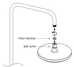
Remove the protective cap from the showerhead ball joint and screw the unit onto the overhead arm ensuring the filter washer is in place.
