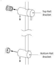
Check the grub screws are wound out. Push the rail brackets onto the top and bottom rail connectors until they are against wall. Secure with grub screws.
