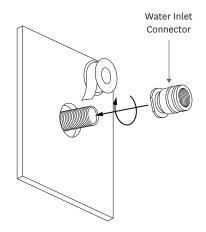
Apply thread tape (or similar) to the 1/2" connection, then screw the top rail connector to the connection.
