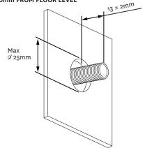
Install a ½" male threaded connection at the recommended height on wall, ensuring that a minimum of 10mm of thread protrudes past the finished wall.
