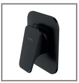
CONSTRUCTION: Brass body CARTRIDGE TYPE: Ceramic CLASSIFICATION: Suitable for all pressure systems INLET CONNECTIONS: 1/2 " BSP Male OUTLET CONNECTIONS: 1/2 " BSP Male WORKING PRESSURE: 35 - 500kPa OPERATING TEMPERATURE: 5 °C - 80 °C  Fastflow™ technology incorporated for unrivalled performance on unequal pressure
