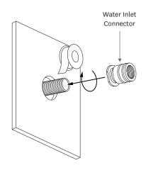
Apply thread tape (or similar) to the  $\frac{1}{2}$ " connection, then screw the top rail connector to the connection.
