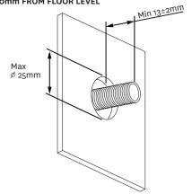
Install a 1/2" male threaded connection at the recommended height on wall, ensuring that a minimum of  $13\pm2$ mm of thread protrudes past the finished wall.
