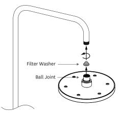
Remove the protective cap from the showerhead ball joint and screw the unit onto the overhead arm ensuring the filter washer is in place.
